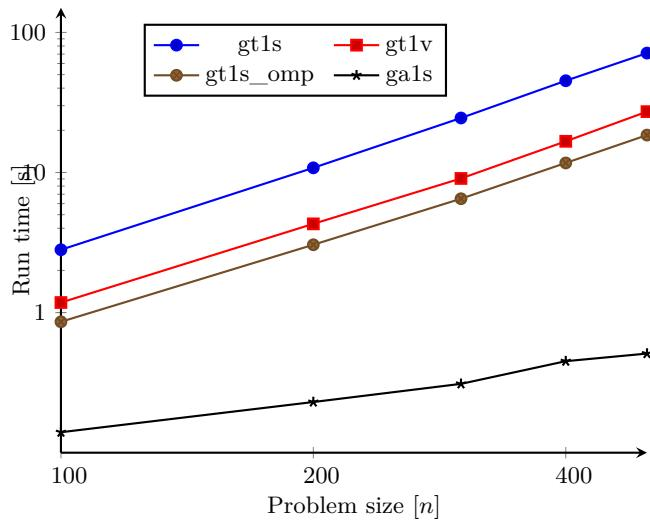
**Abbildung 3.** Race: We compare run times (in seconds) for gradients of the midpoint of the solution of Burgers' case study with respect to the initial condition for  $m = 1000$  implicit Euler steps and  $n = 100, \dots, 500$  spatial grid points. Four `dco/c++` modes are considered: Scalar tangent mode (`gt1s`), vector tangent mode with vector length  $n$  (`gt1v`), parallel scalar tangent mode with OpenMP on four threads (`gt1s_omp`), scalar adjoint mode (`gals`).
