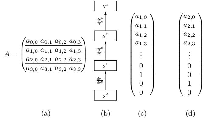
**Abbildung 9.** Parallel accumulation of two inner rows of the Jacobian  $A \in \mathbb{R}^{n \times n}$  (a) for the Burgers case study with  $n = 4, m = 3$  and using two threads: Tape of evolution of state with preaccumulated local Jacobians of individual time steps (b); second row computed by first thread using vector of scalar adjoints (c); third row computed by second thread using vector of scalar adjoints (d).
