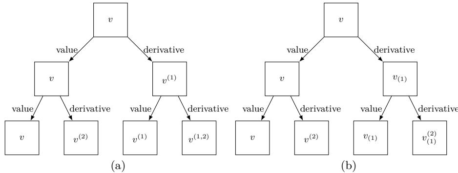
**Abbildung 4.** Data access in second-order (tangent over) tangent (a) and (tangent over) adjoint (b) types provided by `dco/c++`
