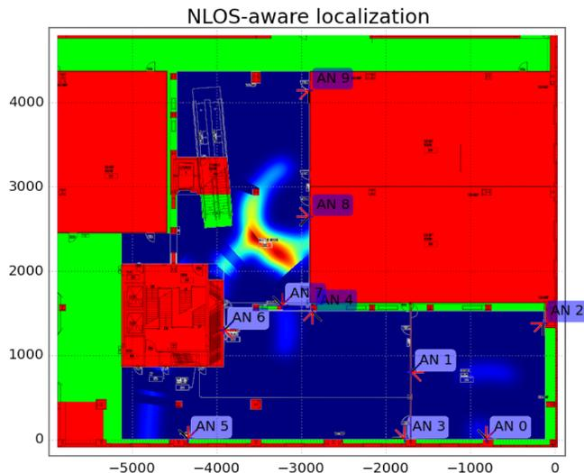
Fig. 2. Relative probabilities of a node’s position as calculated by our current software. Both axes in cm. Reproduced from [6].
