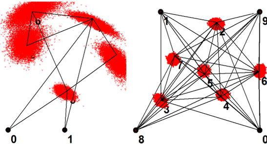
Fig. 2. simulation of effect of range measurement error on calculated node-coordinates with standard deviation of measured ranges of 0.5 length-units. The minimal outer problem exhibited the the highest sensitivity, the full inner problem proved to be most stable.
