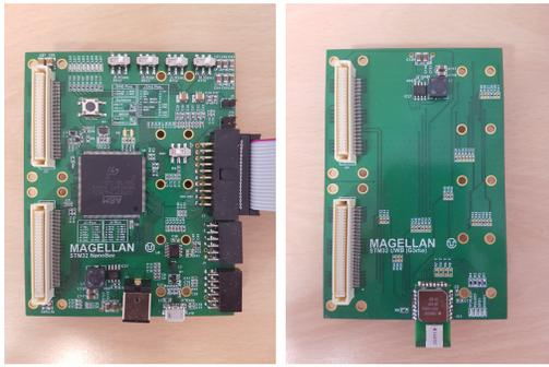
(a) Data processing PCB (b) UWB PCB
