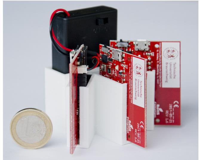
Fig. 1. Anchor node consisting of three INGA sensor nodes. Reproduced from [6].
