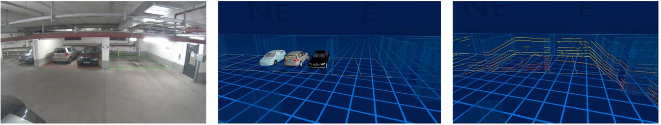
Fig. 2: Three parking lot perspectives: Visual (left), virtual (center), LiDAR scanner (right).
