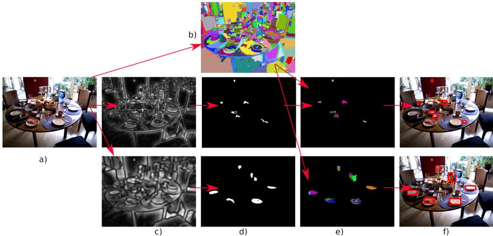
Fig. 2: Object proposal generation: a) original image, b) superpixel segmentation c) for octaves 1 and 2, their specific saliency maps, d) salient blobs obtained by region-growing, e) combining superpixels into object proposals with help of salient blobs, and e) bounding boxes of the object proposals.
