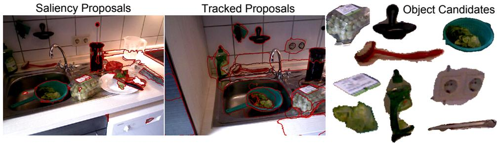
Fig. 1: Overview of our sequence-level proposal detection. Left: proposals from our frame-based, multi-saliency object discovery. Middle: sequence-level proposals from tracking. Right: Visualization of some of the candidate objects.
