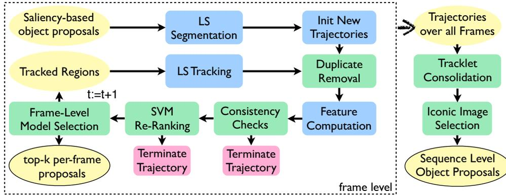
Fig. 3: Overview of the tracking pipeline for obtaining sequence-level proposals.
