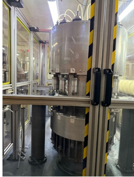
Figure 2: Automated module of the line for applying decoration to caps at the JSC “Technologia” enterprise.
