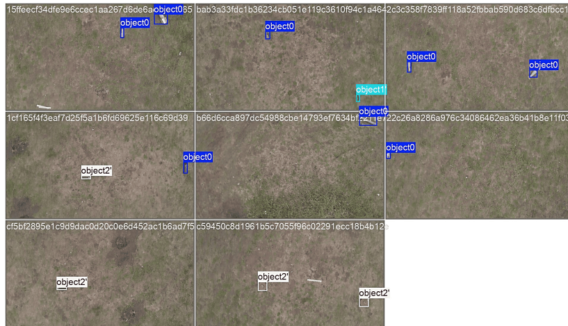
Figure 11: Example validation batch with YOLOv11s predictions (epoch with the best validation metrics). Detected instances of classes object0 , object1 , and object2 are shown together with confidence scores.
