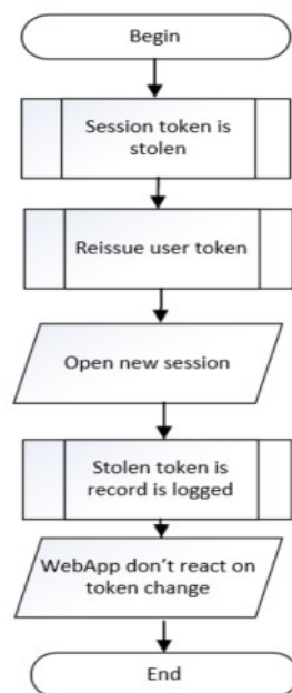
Figure 3: Algorithm for protecting web application from session fixing attacks
