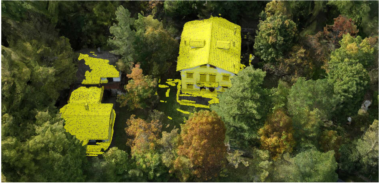
Figure 7: CesiumJS Classification Primitive on building area marked with a transparent yellow overlay
