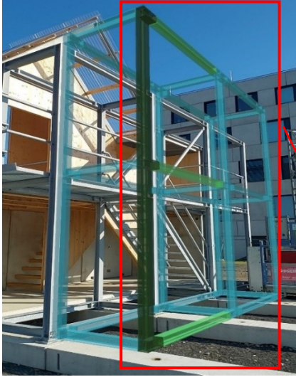
Figure 5: Screenshots of the AR application, showing the construction of another module of the steel frame and its subsequent sub-element with metadata when the mesh is selected.
