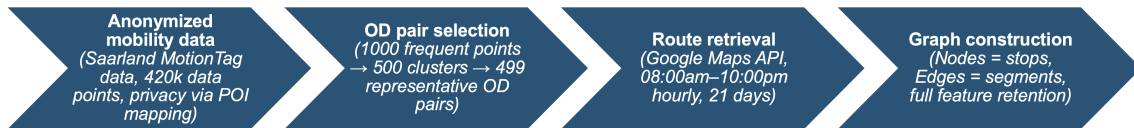
Figure 2: Data processing pipeline for the ROMY rural pilot. Anonymized mobility traces from the Saarland MotionTag dataset (420k points) are privacy-preserved via mapping to public Points of Interest. The 1000 most frequent locations are clustered into 500 groups, yielding 499 representative origin-destination (OD) pairs. For each pair, the Google Maps API is queried hourly (08:00–22:00) over 21 days. Retrieved routes are converted into a directed, attributed graph retaining all spatial, temporal, modal, and semantic features for GNN-based risk estimation.
