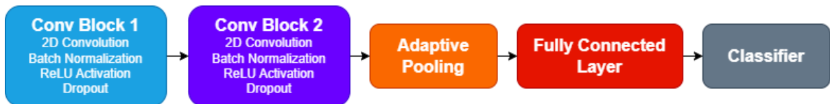
Figure 3: Diagram of Convolutional Neural Network (CNN) to extract features
