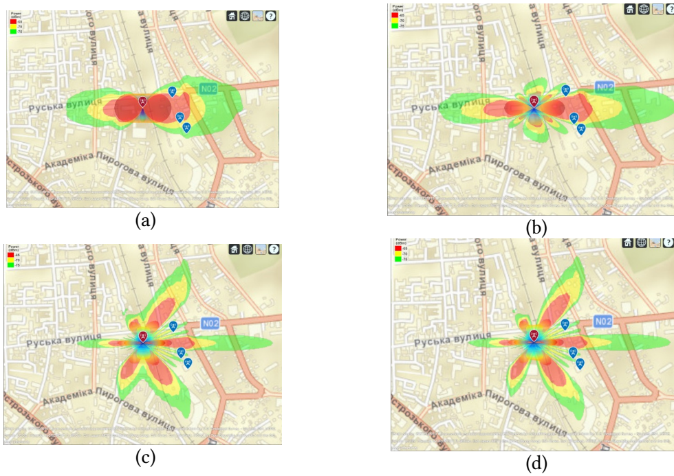
Figure 6: Radiation pattern of the ultrawideband Vivaldi active phased array antenna projected onto the terrain surface for (a) 1.2 GHz, (b) 2.4 GHz, (c) 5.8 GHz, and (d) 5.8 GHz.
