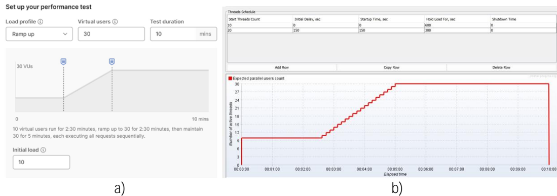
Figure 3: Ramp Up load parameters with 30 VUs and 10 VUs as initial load, test duration 10 mins: a) Postman load profile; b) Ultimate Thread Group plugin configuration in JMeter.
