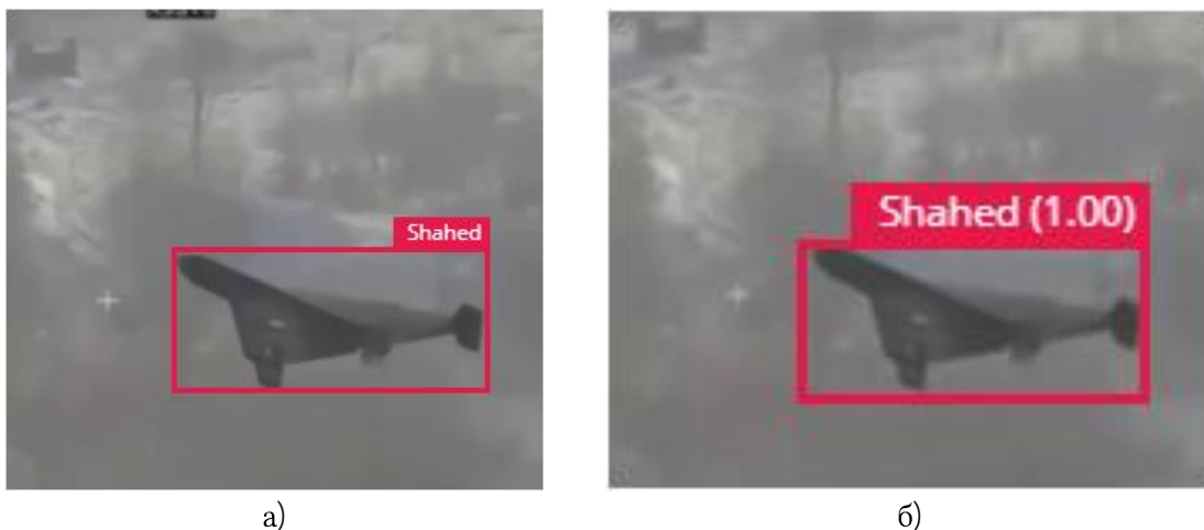
Figure 2: a) Video frame with Shahed-136 image, and b) probability of object detection with MobileNetV2 SSD FPN-Lite model
