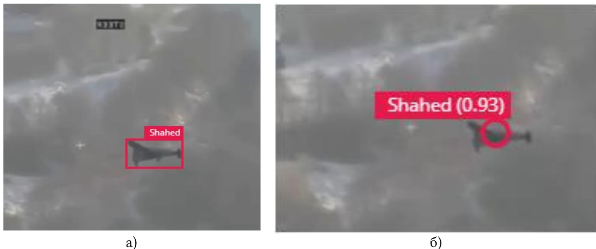
Figure 3: a) Video frame with Shahed-136 image, and b) probability of object detection with FOMO model
