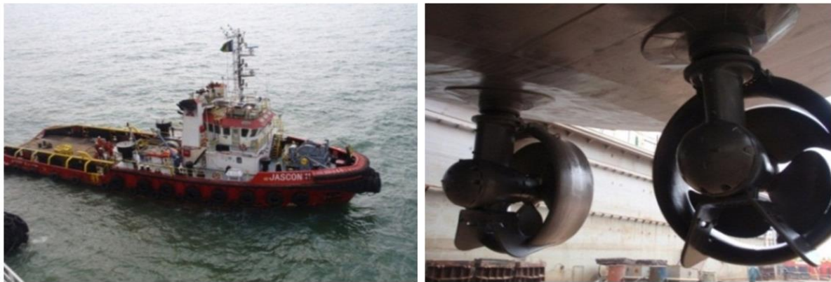
Figure 1: Anchor handling tug AHT Jascon 11 (IMO 9386847) and its stern azipods.
