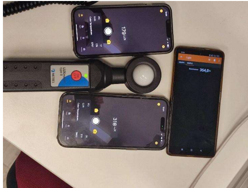
Figure 6. Phone sensor value comparison with reference Metrel Eurotest 61157 device
