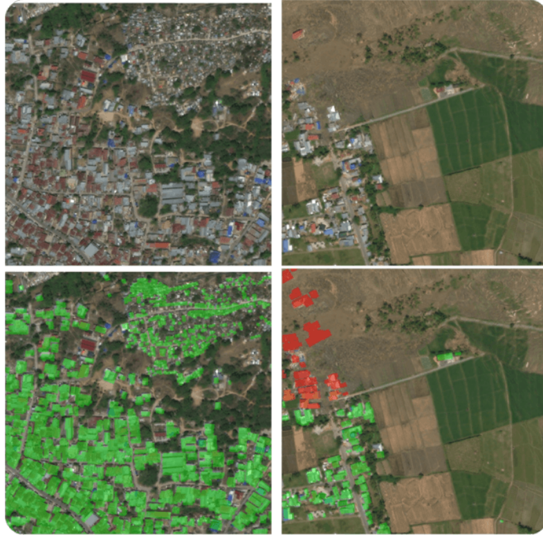
Figure 3: An example of post-disaster images that show damaged areas with colours: green for minor damage, orange for significant damage, and red for destroyed [32]
