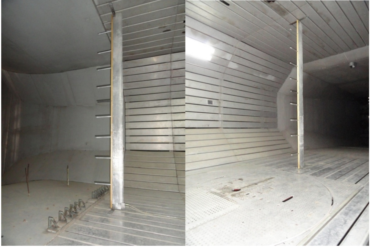
Figure 1: The comb in the working part of the wind tunnel (at the section of the nozzle and inside the wind tunnel).
