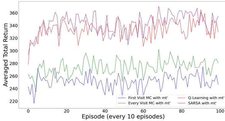
**Figure 3:** The total returns obtained using different algorithms with a changing epsilon ( $mt'$ ). The x-axis and y-axis represent the count and average total return, respectively, per 10 episodes. The initial epsilon for all the algorithms is 0.1 and the learning rate for Q-Learning and SARSA is 0.25.
