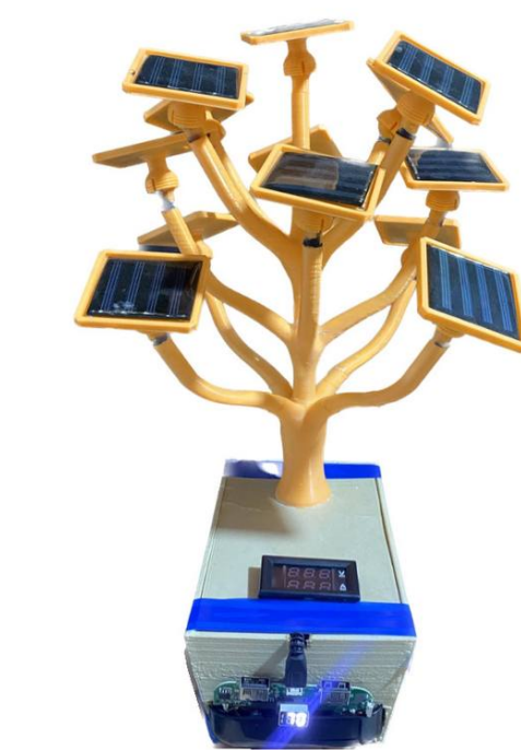
Figure 10: The final form of the solar tree
