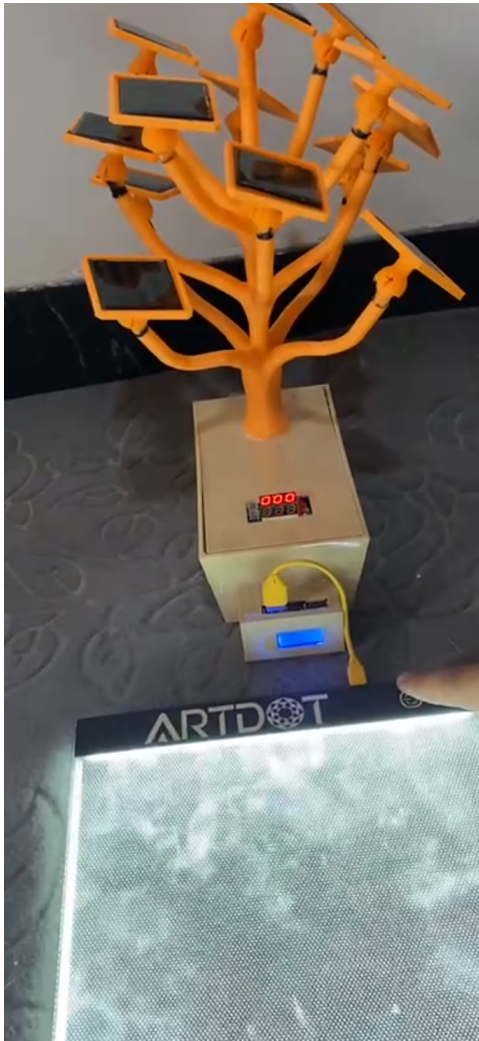
Figure 12: Powering the Light Pad using the solar tree
