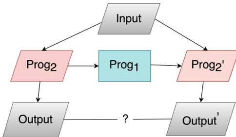
**Figure 1:** Traditional refactoring.  $Prog_1$  is the refactoring.  $Prog_2$  and  $Prog_2'$  are programs to be refactored and the refactored program, respectively.  $Output$  and  $Output'$  are the outputs of  $Prog_2$  and  $Prog_2'$ , respectively, given  $Input$ . Assume  $Prog_2 \neq Prog_2'$ .
