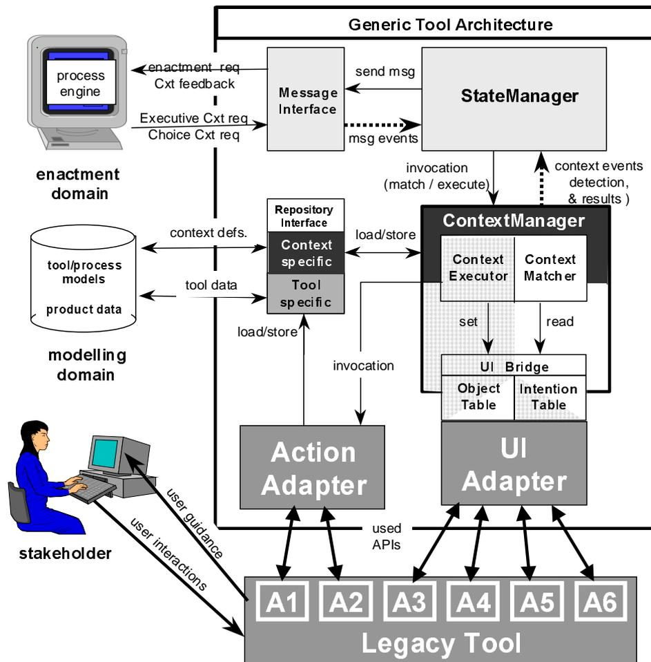
Figure 13: Adding adapter layers to the generic tool architecture for integrating legacy tools.
