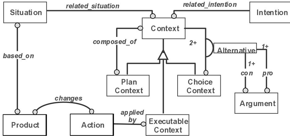
Figure 3: The NATURE process meta model [47], [66].
