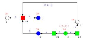
**Fig. 3.** CPN model for cells linked in a pipeline. The declarations are as follows: colourset CS = int with 1 - N, variable x: CS. The arc expression [x > 1] - x indicates that the first cell is not linked to the last, meaning cells are linked in a linear pipeline.
