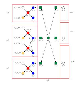
Fig. 5. Refined Petri net model for a single cell with seven compartments (labelled vc1, vc2,..., vc7). Each place or transition belongs to a specific compartment, indicated by a number given as a suffix in place or transition names. NW and SW denote two left neighbours of the current cell.
