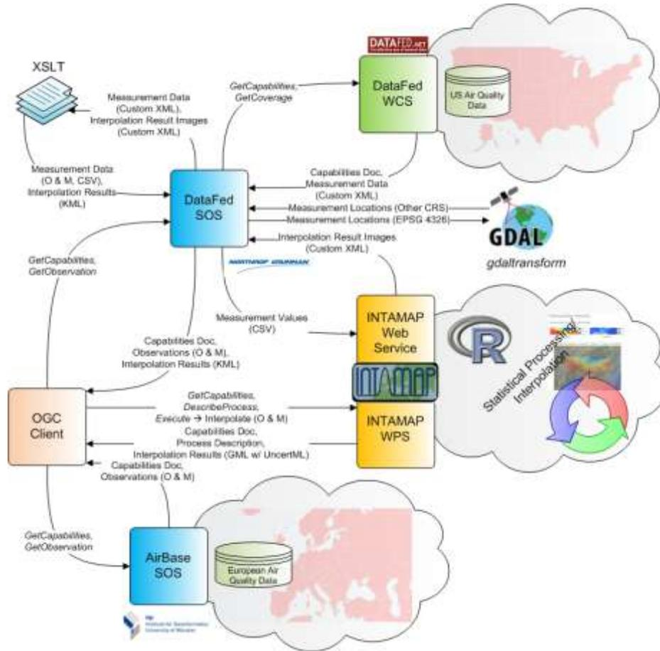
Fig. 1. Interpolation System Architecture
