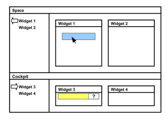
Fig. 1. Conceptual user interface of a PLE with inter-widget communication, displaying two widgets in a space and another two widgets in a cockpit, where a widget in the space is broadcasting an event that is accepted by a widget in the cockpit.
