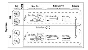
Fig. 1. Two Level Assisted MAS Architecture(2-LAMA): Domain Level (DL), Meta Level (ML) and Interface.
