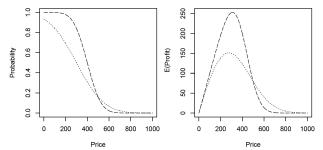
Fig. 5. Probabilistic buying models of 2 different customers approximated by 2 normal distributions with  $\mu_1 = 400$  and  $\sigma_1 = 100$ , and  $\mu_2 = 300$  and  $\sigma_2 = 200$ . Left: Probability distribution function. Right: Associated expected profit.
