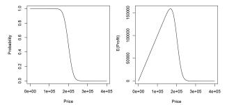
Fig. 2. Probabilistic buying model of a customer approximated by a normal distribution with  $\mu = 200,000$  and  $\sigma = 20,000$ . Left: Probability distribution function. Right: Associated expected profit.
