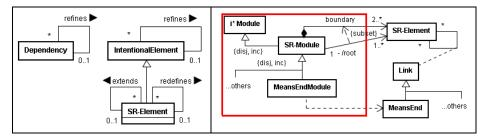
Fig. 2. Extending the *i*\* metamodel, excerpts: inheritance (left) and modules (right).
