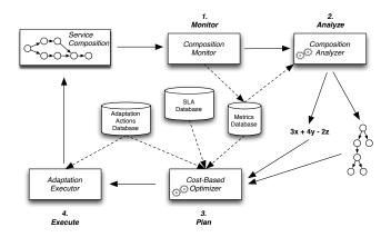
Fig. 1: A Self-Optimizing System for Cost-Optimal SLA Conformance
