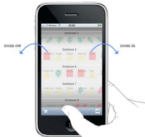
Figure 1. The tap hold/tilt interaction technique.
