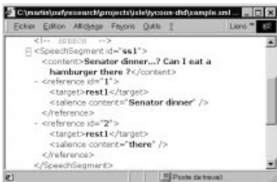
Figure 3: A speech segment (“Senator dinner ... ? can I eat a hamburger there ?” which contains two references.
