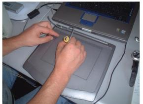
Figure 2. Experimentation of the AudioTact<sup>™</sup> device: a visually impaired user explores the virtual image using the left hand for spatial references and the right hand for scanning for aural and vibrational cues.
