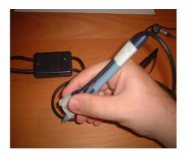
Figure 1. Experimentation of the AudioTact<sup>™</sup> device: a picture of a pen with the vibro-audio device attached.
