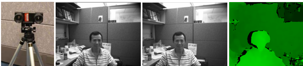
Figure 1 (a) Stereo video camera. (b) Left image. (c) Right image. (d) Disparity map d(x,y) produced by stereo algorithm: brighter green means higher disparity and thus closer to camera; black pixels indicate no estimate at that location. The disparity map clearly shows that the person in the images is closer to the camera than the walls behind him.
