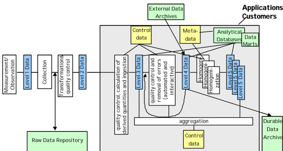
Figure 1: Schematic representation of the process chain/life cycle for processing meteorological data (adapted from [Konzelmann 1998]). The large rectangle area denotes the parts of the process that are covered by the data warehouse system.
