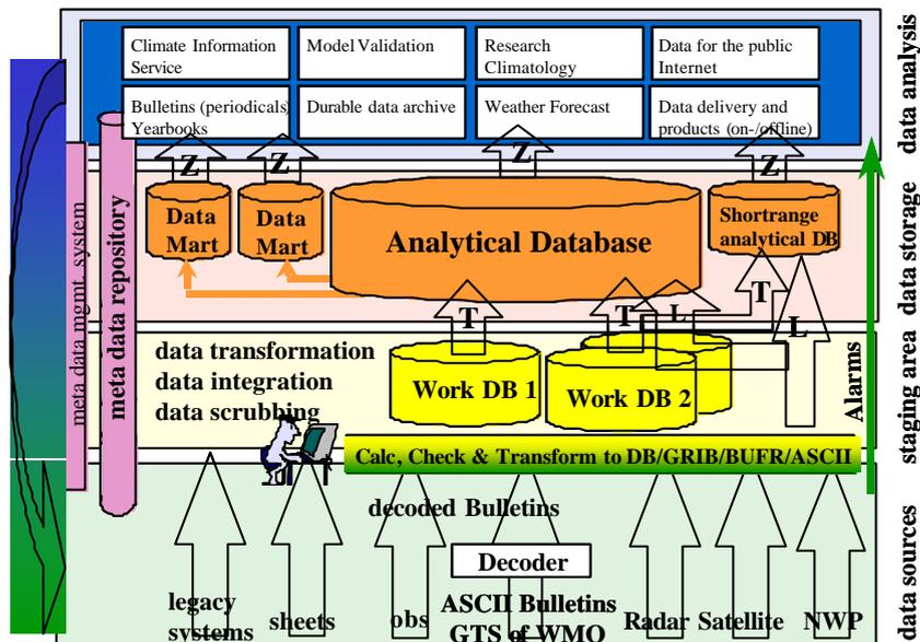
Figure 2: Conceptual architecture of the MeteoSwiss data warehouse system. Arrows depict data flows (T - transformation and loading, L - loading without transformation, Z - ad hoc queries).
