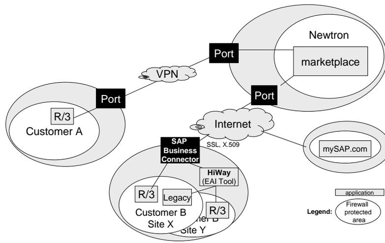
Figure 3.4-3: Technical view on intermediate solutions
