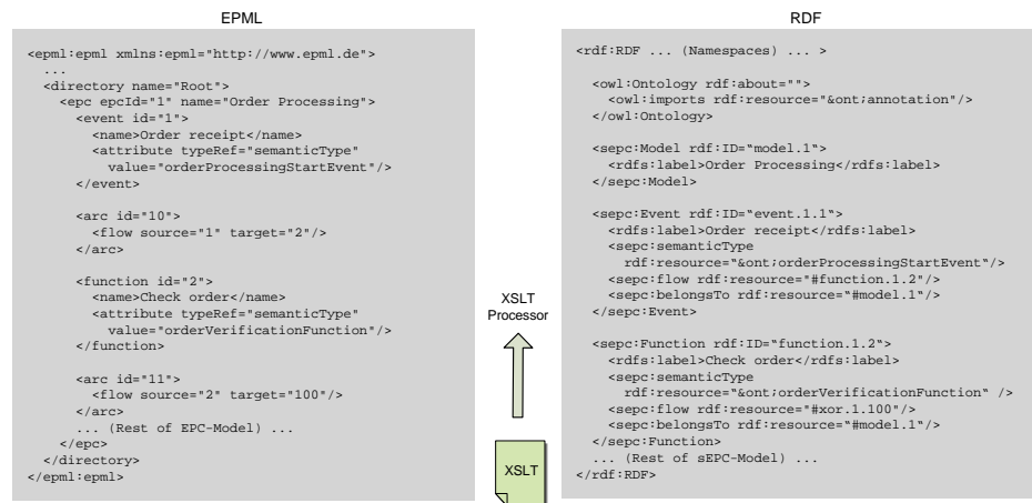
Fig. 7. Transformation from EPML to RDF
