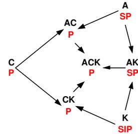
Fig. 4. Sheaf representation of the sensors  $A, C, K$  informing the variable  $P$ . The arrows are functions transforming data on faces into a common form.
