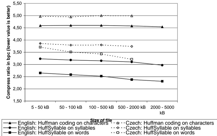
**Fig. 2.** Comparison of Huffman-based methods on English and Czech texts
