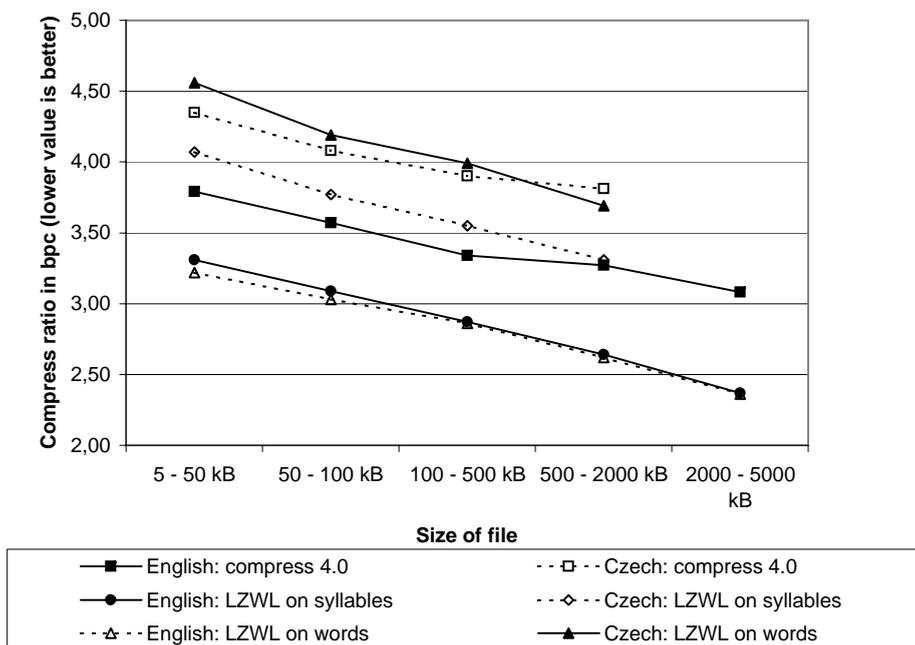
Fig. 1. Comparison of LZW-based methods on English and Czech
