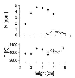
Fig. 1: T and  $f_v$  axial profile in  $C_2H_4$  (closed diamonds) and  $CH_4$  (open circles) diffusion flames
