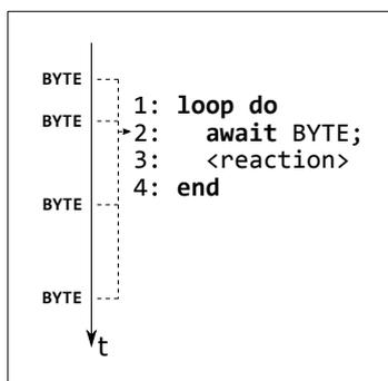
Figure 4.5: Programming scheme of the single entry point model
