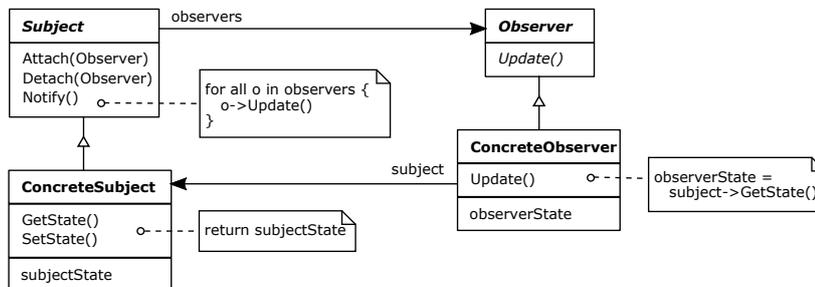
Figure 5.10: Structure of the *Observer* pattern [Gam+95]
