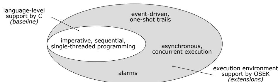
Figure 4.3: Underlying technologies provided by C and OSEK
