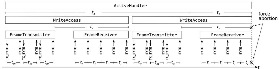
Figure 5.6: Hierarchical timing constraints for fieldbus communication
