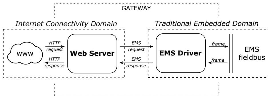
Figure 3.1: Top-level view of the gateway's system architecture
