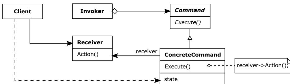
Figure 5.7: Structure of the *Command* pattern [Gam+95]
