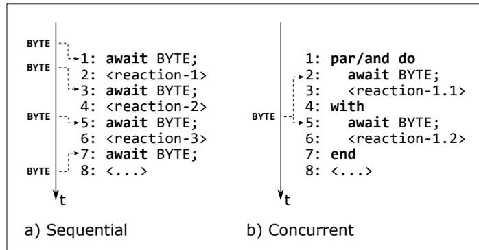
Figure 5.5: Programming scheme of the multiple entry points model in CÉU
