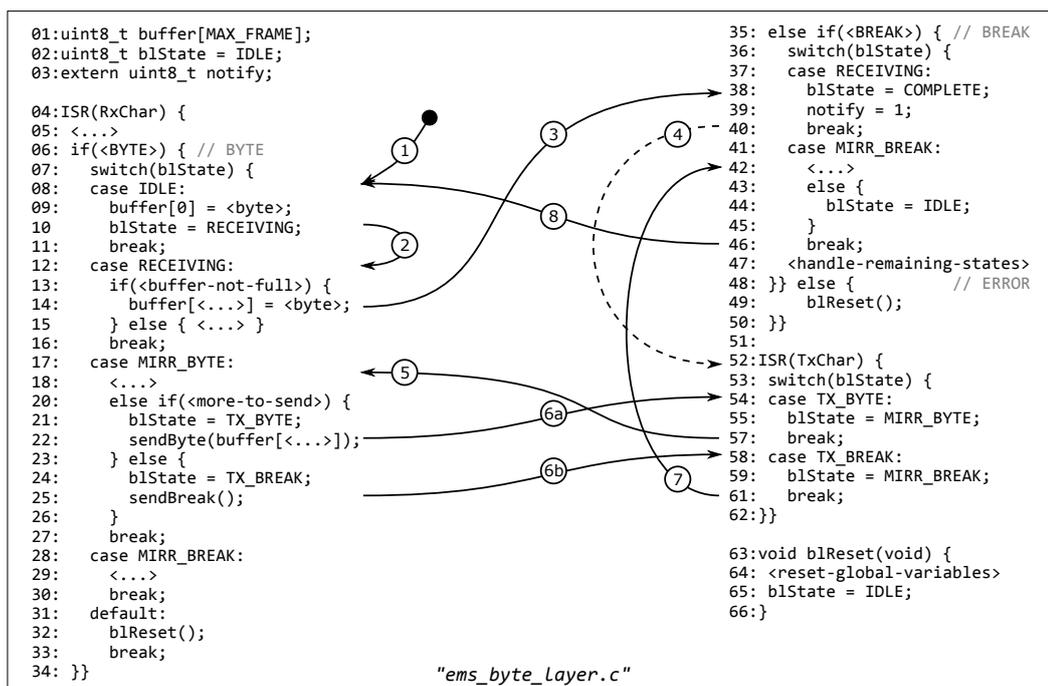
Figure 4.6: Outline of the byte layer implementation featuring  $\text{Receive}_{\text{BL}}$  and  $\text{Transmit}_{\text{BL}}$  (arrows 1 to 8 depict the logical control flow performed for one run of  $\text{Respond}_{\text{FL}}$ )
