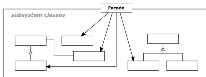
Figure 5.8: Structure of the *Facade* pattern [Gam+95]
