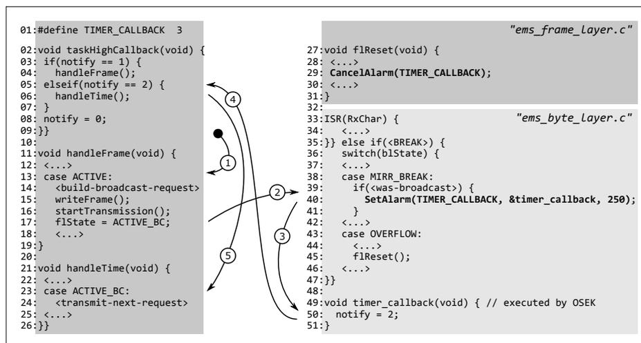
Figure 4.13: Outline of a delay implementation in C
