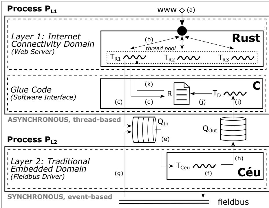
Figure 5.2: Domain-oriented, layered software architecture with CÉU and RUST
