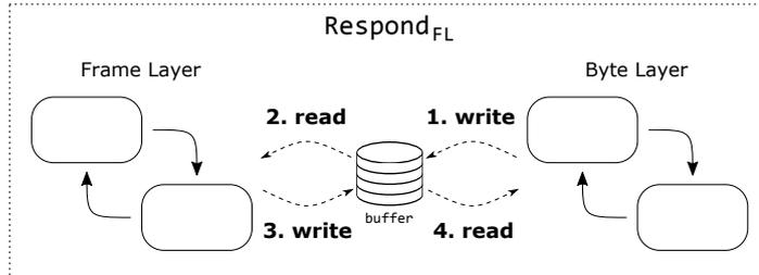
Figure 4.10: Order of accesses to `buffer` required for `Receive_BL`
