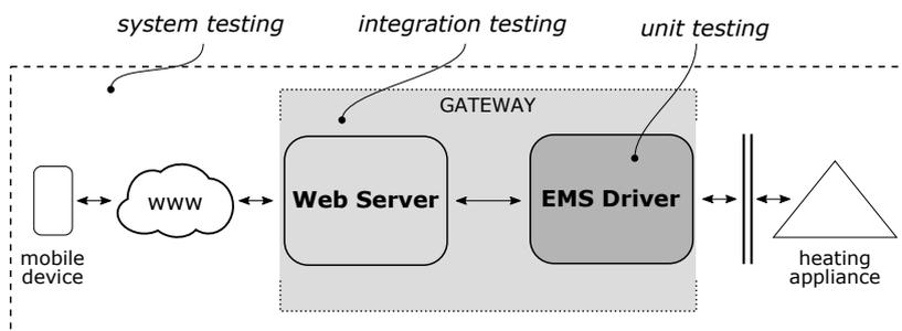
Figure 5.12: Test classes for the gateway application
