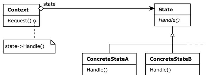
Figure 5.9: Structure of the *State* pattern [Gam+95]
