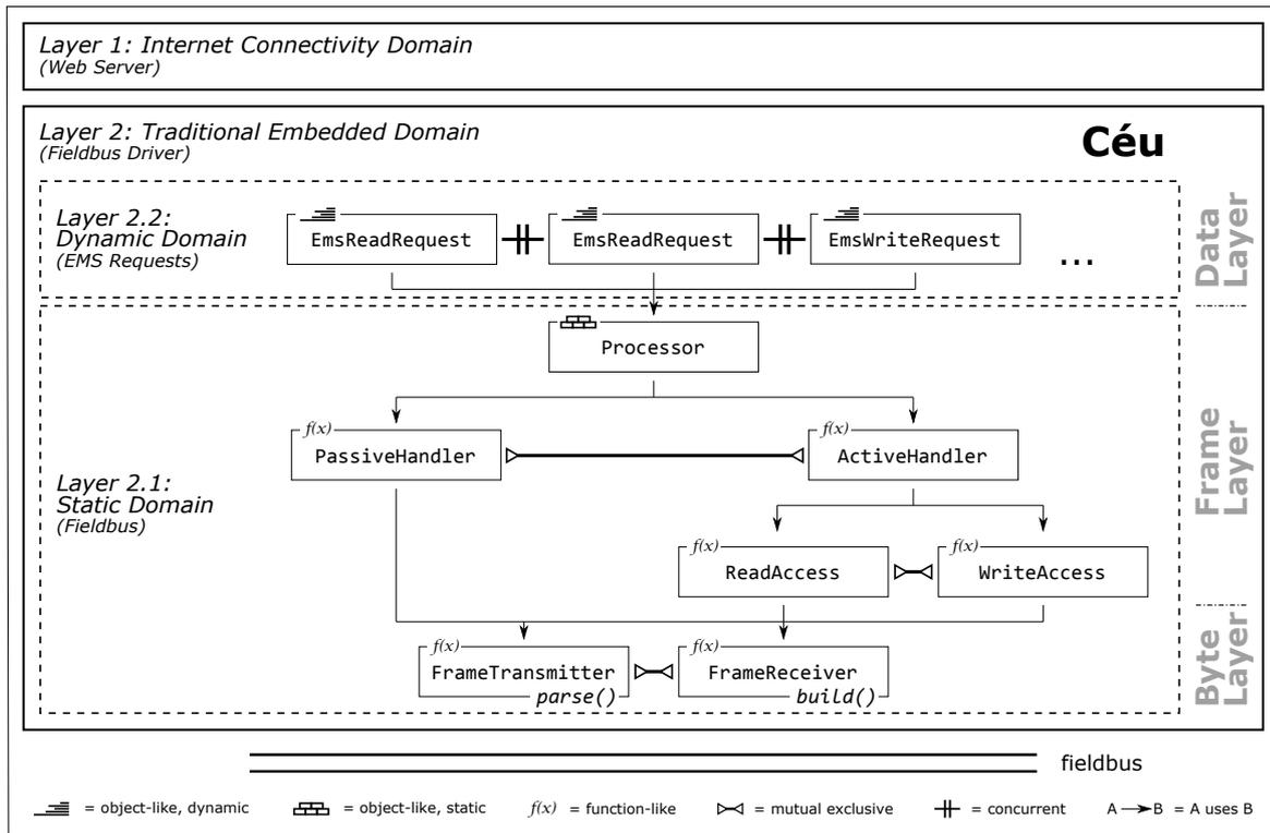
Figure 5.4: Layered architecture of the fieldbus driver in CéU
