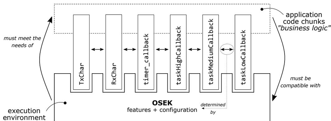
Figure 4.15: Dependency between application code and execution environment
