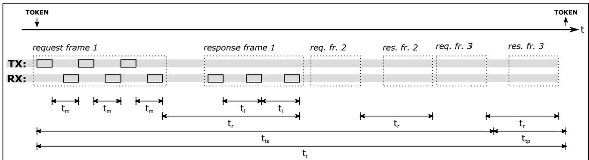
Figure 2.2: Fieldbus communication time intervals of a slave in Active Mode (TX: outgoing bytes, RX: incoming bytes)
