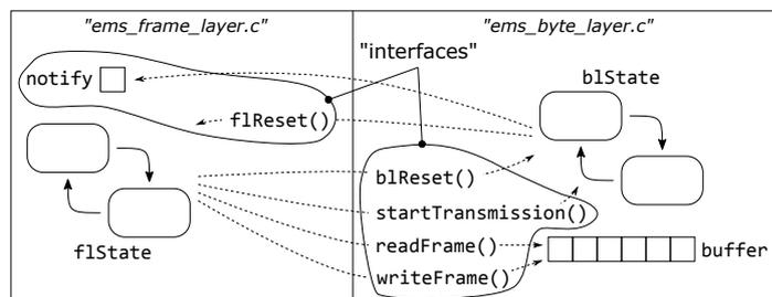
Figure 4.9: Interaction between byte and frame layer
