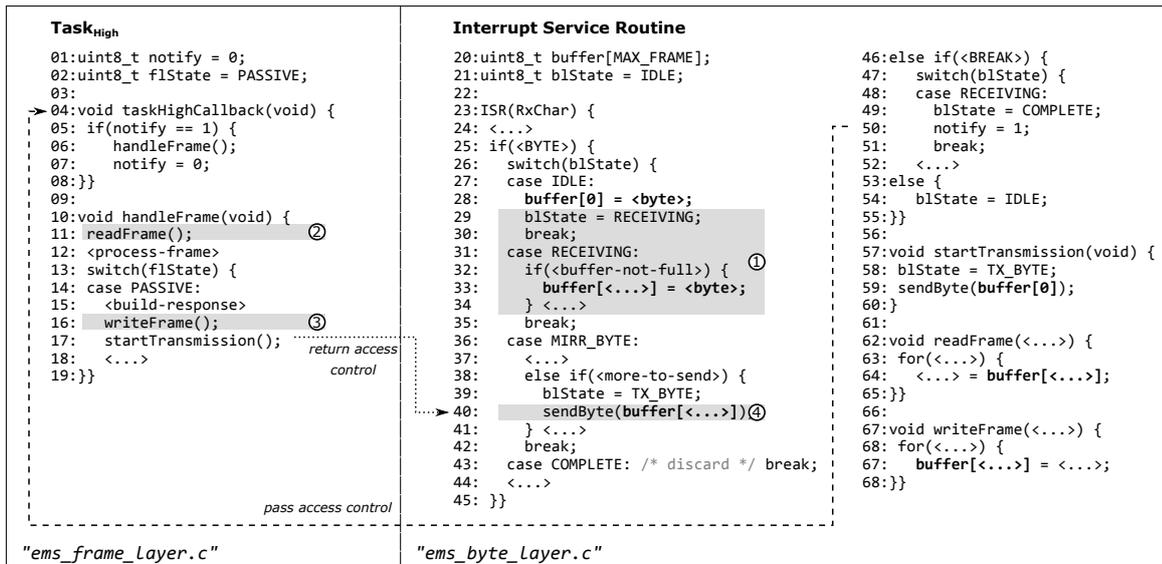
Figure 4.11: Synchronization without operating system support in C
