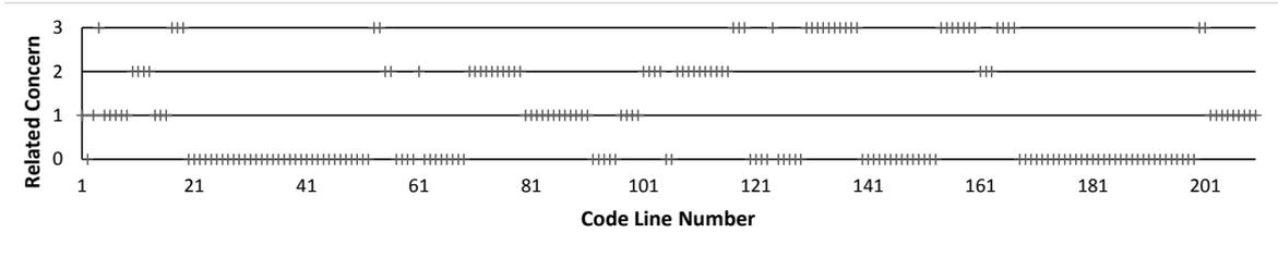
Figure 6.1: Mapping between routine RxChar code line and communication concern in the C implementation: Transmit<sub>BL</sub> (3), Receive<sub>BL</sub> (2), both (1), other (0).
