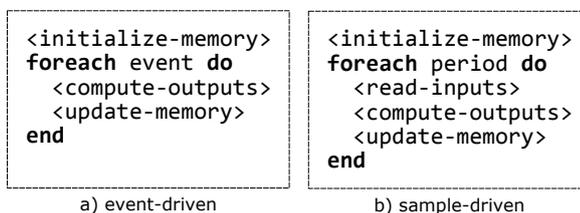
Figure 2.3: Two common synchronous execution schemes [Ben+03, p. 65]
