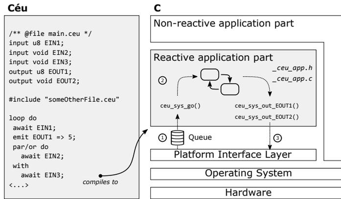
Figure 2.5: System integration of CÉU code
