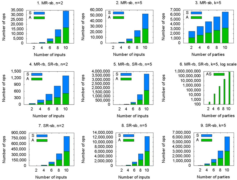
**Fig. 7.** Number of basic homomorphic ( $A$ ), homomorphic scalar ( $S$ ) operations or both in sum ( $AS$ ) for *one* party with  $c = n - 1$  in the worst case. (1-3) show results for MR-sb, (4-6) for MR-rb, SR-rb, and (7-9) for SR-sb in cases  $n = 2, n = 5, k = 5$ .
