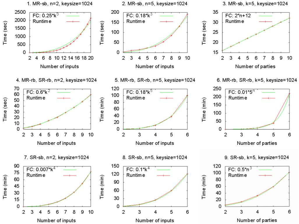
**Fig. 8.** Worst case runtime results with  $c = n - 1$ ,  $l = 1024$  for all MPROS protocols. (1-3) show results for MR-sb, (4-6) for MR-rb, SR-rb, and (7-9) for SR-sb in cases  $n = 2, n = 5, k = 5$ .
